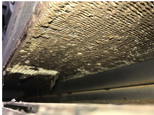
This driver evaporator needs a cleaning!
