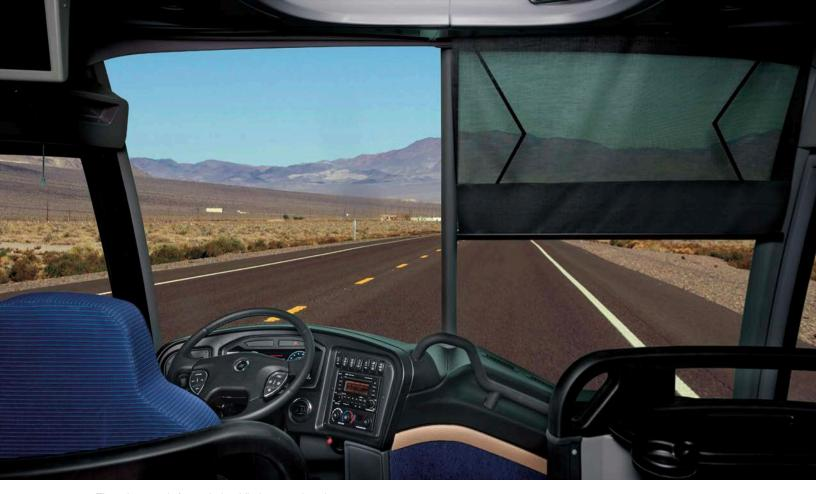
The scissor-style front window blinds recess into the redesigned front cap and blend aesthetically with the parcel racks to improve the panoramic view for passengers.
