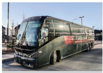
The J4500 CHARGE<sup>TM</sup> provides speeds of up to 72 miles per hour and has a range of 200 miles on a single charge. Other features include regenerative braking to recharge the battery system while braking and the ability to fully recharge the coach in four hours.
