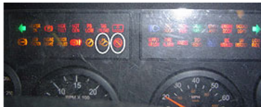
Photo 1 - Check Engine/Stop Engine Tell-Tale lights
